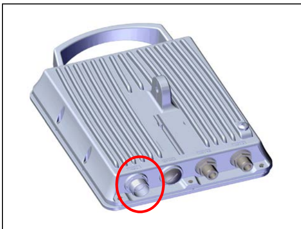
Figure 2-42: Input port: LFF unit (connection label: "IDU")
