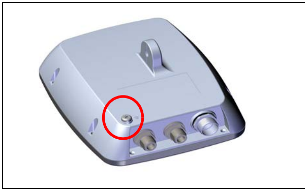
Figure 2-35: Ground: SFF radio unit
