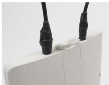
Sealing tape applied
