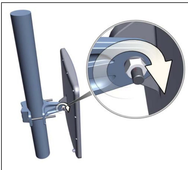
Figure 2-59: Tighten bolt (SU PRO/AIR INT shown)
