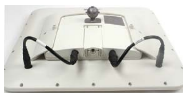
Tape applied on Turbo Gain - 2
